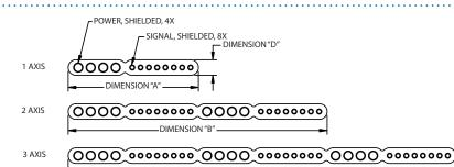
**DIMENSIONS** (inches) WIRE GAUGE POWER В D POWER SIGNAL MIN. BEND А C 1 AXIS 2 AXIS 3 AXIS RADIUS RATING AWG AWG 1KW .846 1.682 2.518 .101 22 28 1″ 1.4" 2KW .950 1.890 2.830 .137 18 28 2″ 3KW 1.098 2.186 .194 14 28 3.274
