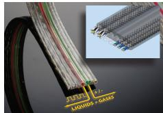
StripMount™ – A reinforced strip, integral to the cable, allows for quick and easy cable mounting, eliminating the need for bulky, expensive cable management systems. The patent-pending StripMount™ feature allows fasteners to be safely inserted through the cable for secure attachment to virtually any surface.
