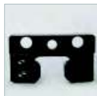
End seal in good condition
