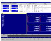
PMAC-NC Pro2 - a Windows-based customizable GUI for PC based CNC control
