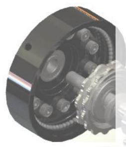
The first track of the cycloidal cam lobes/teeth engage with cam followers located in the reducer housing. Cylindrical cam followers act as teeth of the internal gear. The number of cam followers exceeds the number of cam lobes/teeth.
