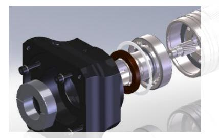
The sun gear is attached to the input shaft which connects directly to the servo motor.
