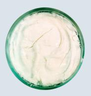
In an oven at 232 °C (448 °F) for 40 hours, Krytox® lubricant had 0% weight loss.
