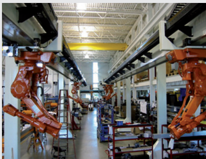
TMO-52-R (ceiling mounted) with an ABB IRB 2400 robot
