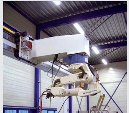
TMO-52-W (wall mounted) with an OTC robot AX-MV4L for welding application
