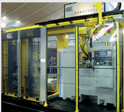
TMO-72 special (45° mounted) with a Fanuc robot M710iC/70T
