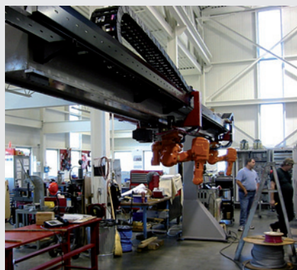
TMO-40-R (ceiling mounted) with an ABB 140 robot
