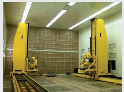
special system, robot lifter for painting application with Fanuc robots
