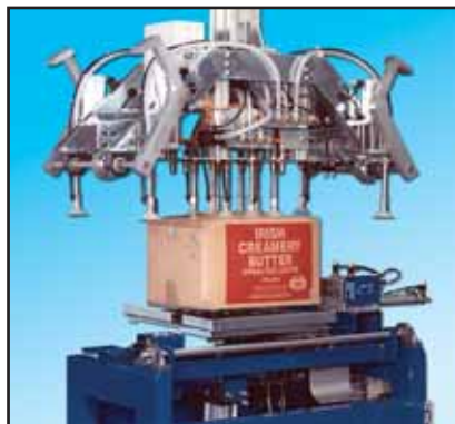
Variable suction gripper for different container
