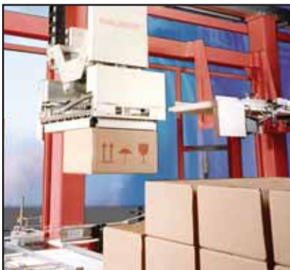
Combined outside suction gripper here carton boxes
