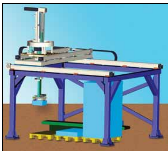
Pallet handling robot with 3 stations.
