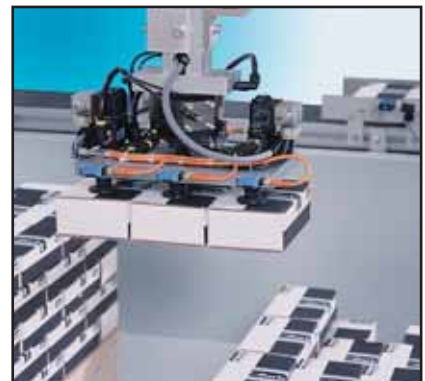
Variable suction gripper for different container
