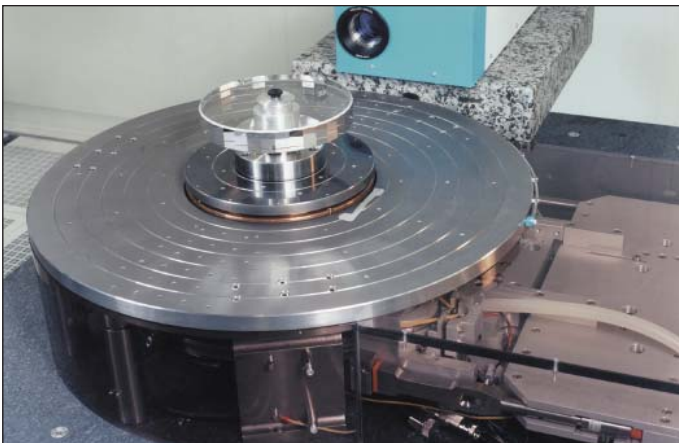
Angle comparator, measuring step approx. 0.001"
