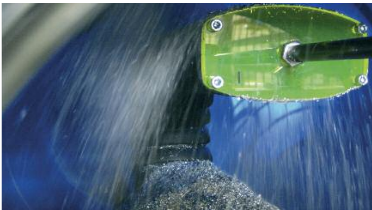
Chip-test at the igus® test-lab proven enormous tightness.
