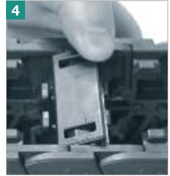
4 Position crossbars. Push down and snap in
