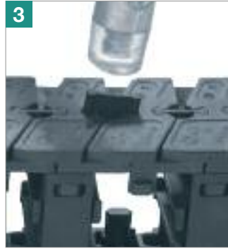
3 Gently insert connector by using a hammer
