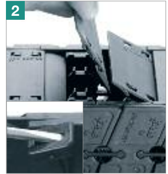
2 ... and remove lids by hand
