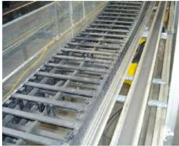
The igus® aluminum "SuperTrough" has been tested since 2005. Test "Axis 1": Speed 4.92 ft/s (1.5 m/s), Travel: 59 ft (18m), Mileage to date: approximately 31,069 miles (50,000 km)
