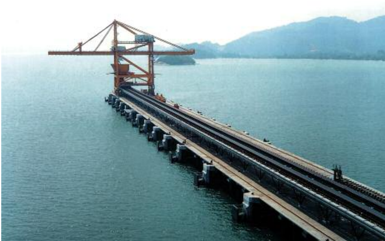
Travel of 1,448 ft. (441.3 m), implemented with igus® Rol E-Chain® Series 5050R
