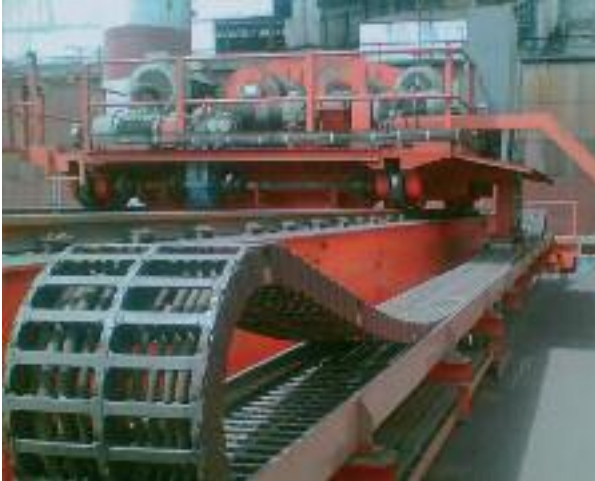
igus® Rol E-Chain® Series 5050R in a steel plant in India with highly corrosive atmosphere - Travel = 22 m, v = 3.28 \text{ ft/s} (1 m/s), a = 3.28 \text{ ft/s}^2 (1 m/s 2 )
