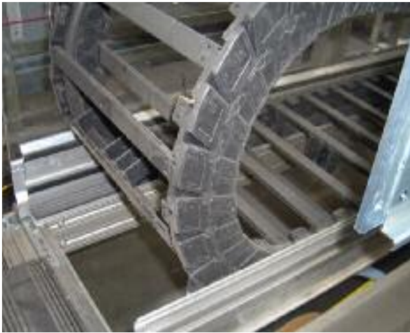
The igus® aluminum "SuperTrough" has been tested since 2005. Test "Axis 1": Speed 4.92 ft/s (1.5 m/s), Travel: 59 ft (18m), Mileage to date: approximately 31,069 miles (50,000 km)
