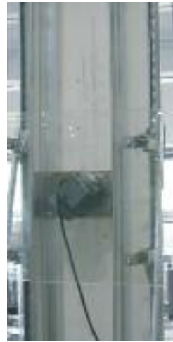
Vibration test: No shifting of trough sections after 108,000,000 rotations at 658 rpm.
