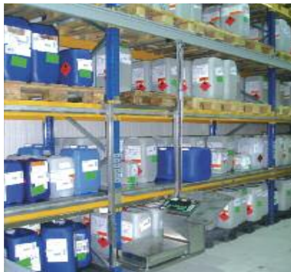
Micro Flizz® as "energy supplying rail guide" for a scale to weigh chemicals, etc.
