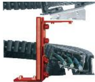
This bottom stanchion (pictured above in red) is required only if the support for the upper run (from a 180° rotation angle) cannot be mounted on the machine.
