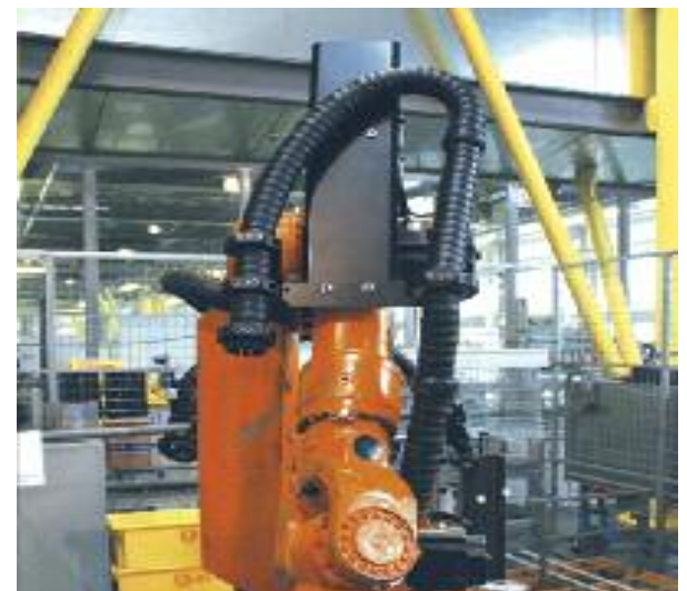
Integrated recuperating spring prevents loop formations
