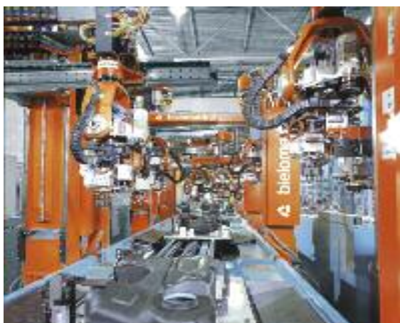
E-Z Triflex® Energy Chains® for multi-dimensional movements on a production line
