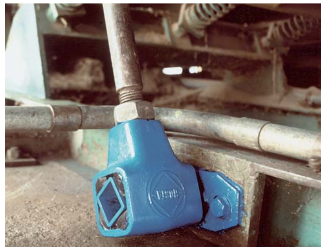
Rocker fixation on feeder frame
