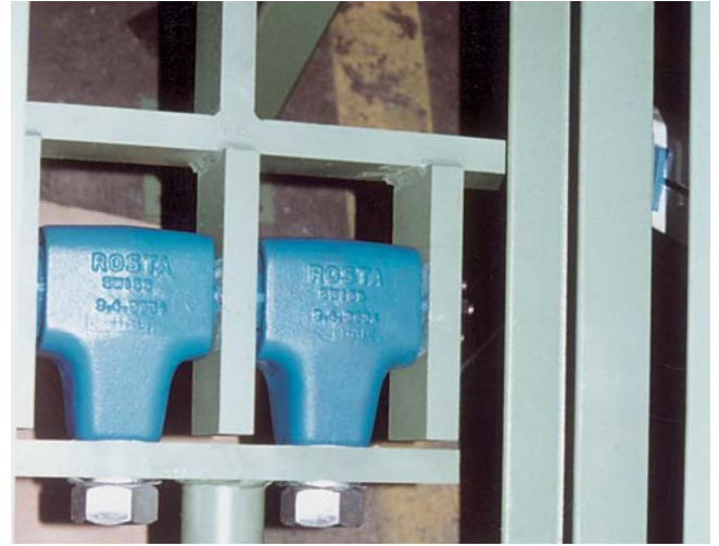
Drive head fixation on chip feeder
