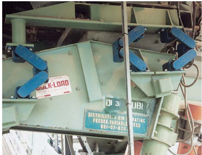
Hanging silo-discharge-feeder on AB
