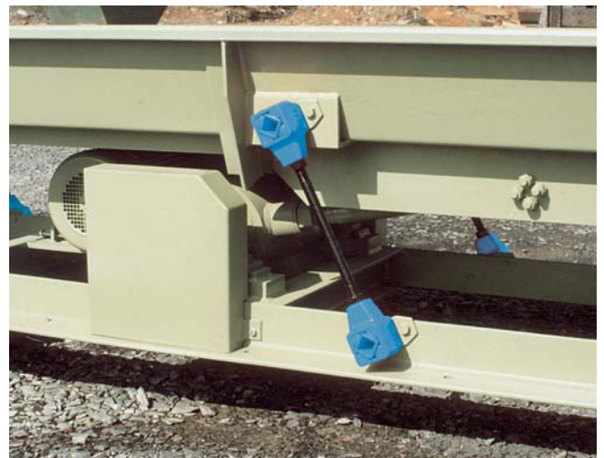
Single rocker on chip feeder
