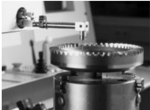
Computerized mapping of gear tooth profile
