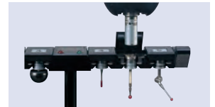
TP200 Compact and high accuracy (stylus change) type
