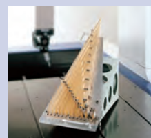
CMM calibration tool using the virtually zero thermal expansion glass gage
