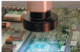
QVP (Quick Vision Probe) For video measurement
