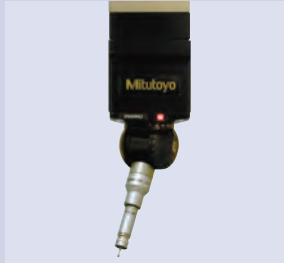
PH10M / PH10MQ Motor drive index type
