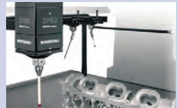
MPP-10 For effective screw depth measurement
