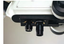
Using optional slide type nosepiece with 2-lens mount (factory set option)
