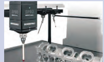
MPP-10 For effective screw depth measurement
