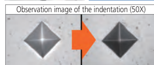
Stray light reduction around the indentation
