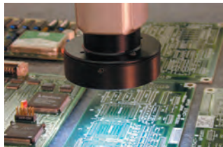
QVP (Quick Vision Probe) For video measurement
