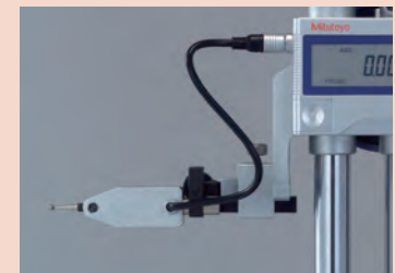
Shown with optional touch-signal probe
