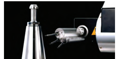
Detector rotation mechanism (0 to 290°, in increments of 1°)
