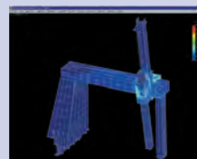
The machine structure has been optimized using FEM (Finite-Element Method) and modal analysis.
