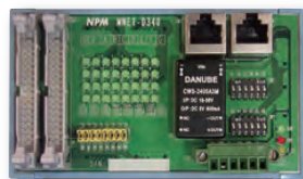
MNET-340 Local Input Board (Isolated 32 inputs)
