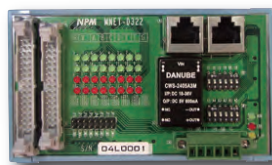
MNET-322 Local Input/Output Board (Isolated 16 inputs/outputs)
