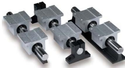
PowerTrax™ Series 100 slide systems are pre-assembled and ready to mount. Series 100 slides consist of combinations of PowerTrax™ Linear Ball Bearing Pillow Blocks, HG shafting, carriage plates and shaft supports. Aluminum carriage plates include threaded steel inserts at key mounting locations. All exposed non-wearing components have a protective, corrosion resistant finish.
