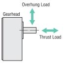
When a chain, gear, belt, etc. is used as the transmission mechanism, the overhung load is always applied on the gearhead output shaft. The overhung load is calculated with the following formula.
