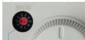
Motor Output Power Select Switch Remove the front panel to access the switch.
