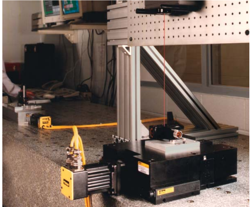
ZP200 utilized in a laser test set-up
