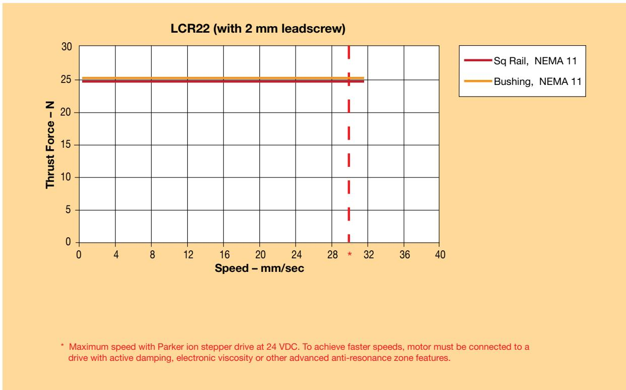
Refer to critical speed limitations on page 7 for specific stroke length maximum speeds.
