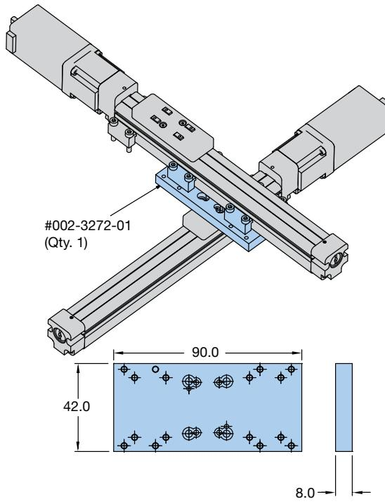
**X-Y Bracket for LCR22/LCR30 Belt-Driven Units**
