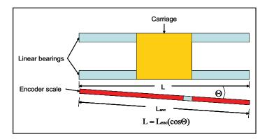
Fig. 18: Cosine errors caused by encoder scale misalignment
