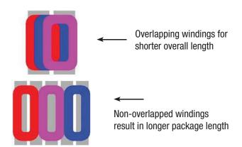
Fig. 9: Overlapping Windings
