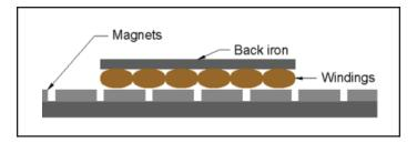
Fig. 13: Slotless Linear Motor
