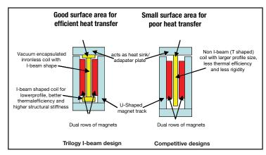
Fig. 10: Parker Trilogy's Patented I-Beam Design
