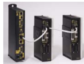
Fig. 17: Parker ACR Controller and Aries Drives
