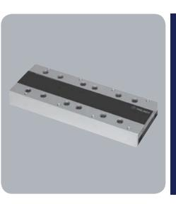
Parker Trilogy's RIPPED ironcore linear motors, with their patent-pending anti-cog technology, can produce the large forces needed for many industrial applications – without the roughness associated with traditional ironcore linear motors. With forces ranging from 13 lbf (57.8 N) continuous up to 1671 lbf (7433 N) peak, the RIPPED family is well suited for a broad range of extremely demanding applications.
