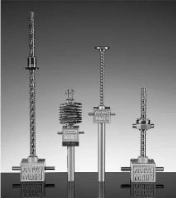
The range of Precision Technology USA, Inc. worm gear screw jacks is comprised of ten models with lifting capacities from 5 kN to 500 kN (5.6 to 56 tons). All versions are designed for both tensile and compressive loads and will operate in any orientation or mounting position.
