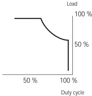
$$F_c = \text{Duty cycle} = \frac{T}{T + R} \times 100$$
