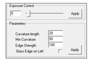
Initial values for "Curvature Length" and "Min Curvature", located under "Parameters", must be entered for Lucana Bead to make accurate measurements. Curvature Length values must be between 10 and 60 while Min Curvature must be between 10 and 100.
