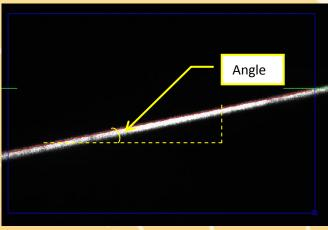
The user interface for Lucana M Tip/Tilt sensor measuring surface tip or tilt of an object or part. The user can view the measurements of tip/tilt in degrees and set the tolerance for pass or fail. The data can be send to another device via UDP, TCP/IP protocol as well as log the data locally or on any network drive.
