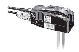
In vacuum chamber applications, the detector head is mounted on the outside of the chamber with the laser beams entering through a suitably positioned viewport. To enable laser alignment to be completed from outside the chamber, this RLD head includes individual pitch and yaw adjusters for both the reference and measurement beams.
