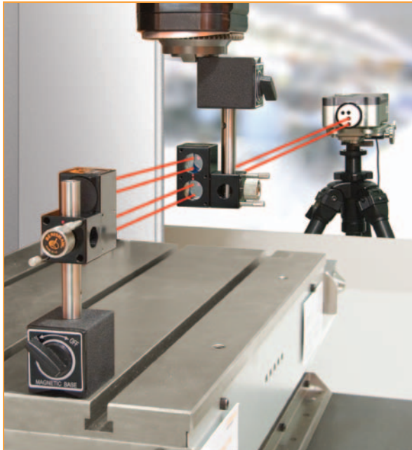
X-axis pitch measurement on a moving bed VMC
