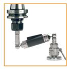
QC20-W wireless ballbar allows rapid condition monitoring of a machine tool's linear axes.
