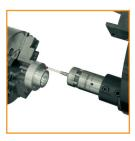
Workpiece inspection probes for automated measurement of component position and alignment.
