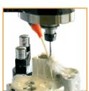
Tool setters enable dynamic setting of cutting tools on the machine tool.
