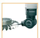
REVO® 5-axis high-speed scanning and multi-sensor inspection system.
