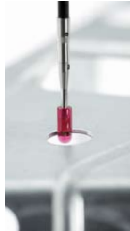
Cylinder styli e.g. for measurement of metal sheets
