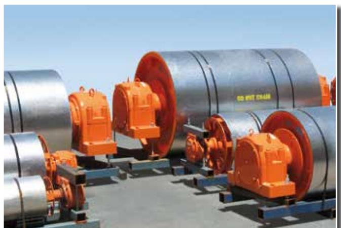
Ready-for-shipping belt drum with Locking Assemblies
