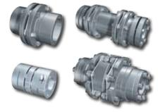
Our torsionally rigid, flexible RING-flex<sup>®</sup> disc couplings can compensate angular, axial, and radial misalignments while transmitting torque in a backlash-free way between driver and driven components. They operate without wear or maintenance, never need lubrication, and, due to their all-metal construction, work well in very high temperatures. RING-flex<sup>®</sup> couplings are pre-engineered to be connected to the shaft with various RINGFEDER keyless locking devices.
