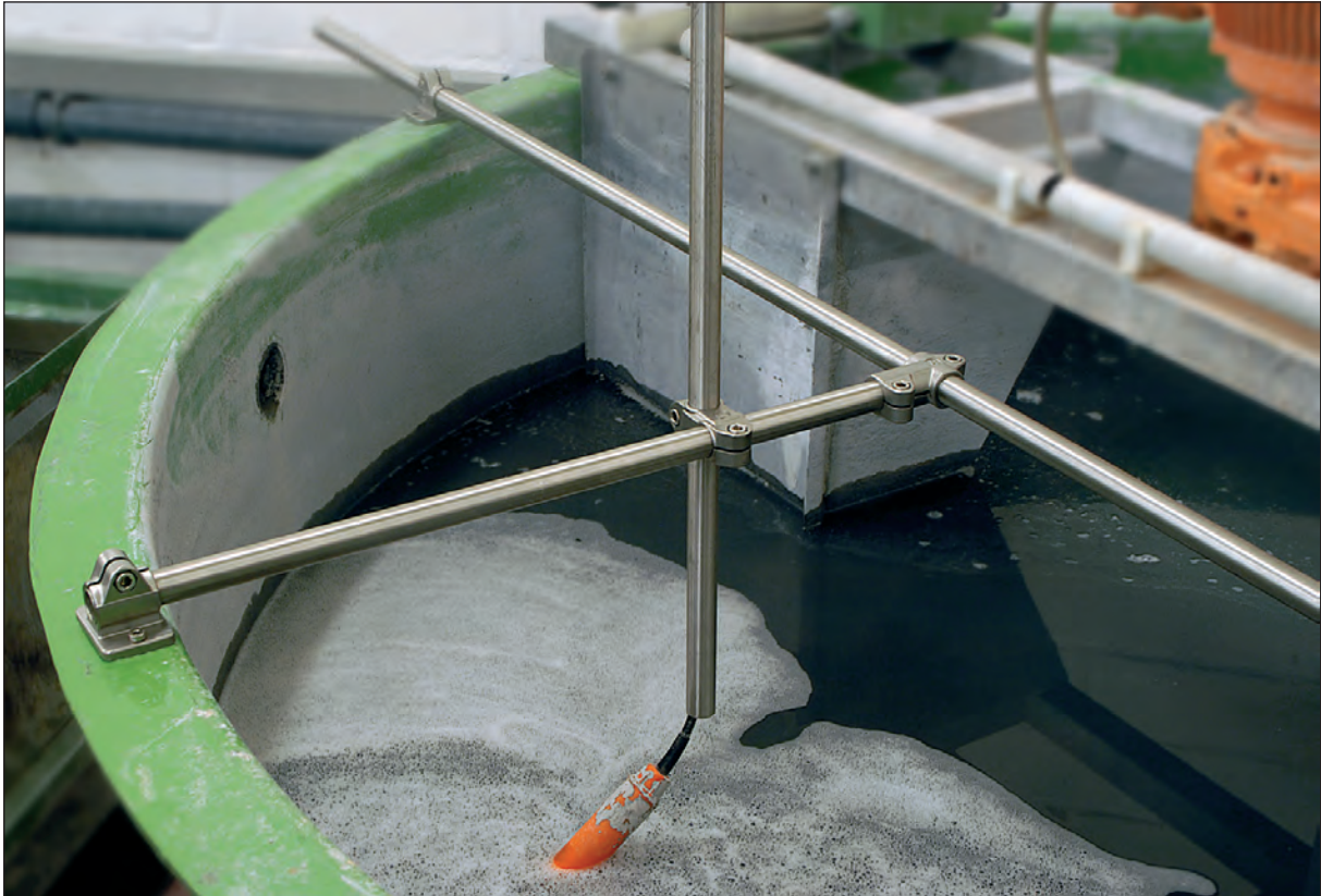
Simple probe fixation in an aggressive environment.
