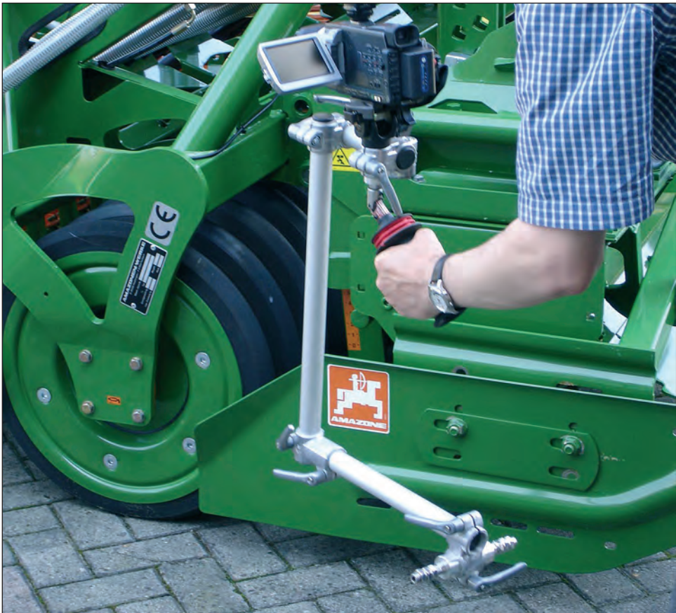
Holder for a camera on a seed spreading machine made of clamping pieces and clamping levers.
