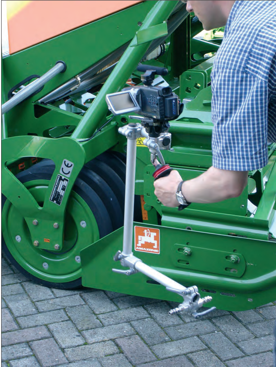
Holder for a camera on a seed spreading machine made of clamping pieces and clamping levers.
