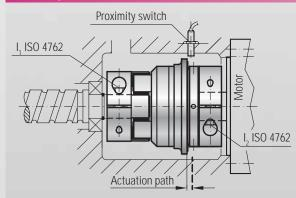
**Mounting:** Slide the coupling onto the respective shafts to the desired axial position. Using a torque wrench, tighten the clamp screws to the correct tightening torque as indicated in the table.
