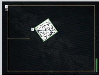
Code reading on solar cells Even extremely small codes, such as those on silicon solar cells, or highly reflective codes, e.g. on thin-layer solar cells, can be read.
