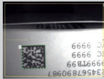
Printed codes on pharmaceutical packaging It is possible to search for both ECC200 or bar codes (e.g. EAN 13) simultaneously. In addition to code reading, the presence of optical characters can be inspected using object detection.
