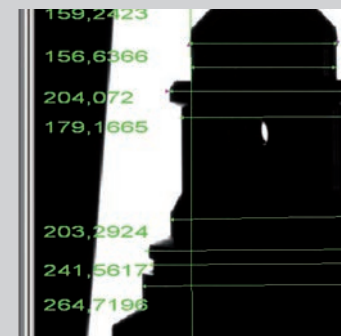
Taking measures: The dimensional accuracy of an object (e.g. a turned or pressed part) is an important quality feature, and can indirectly provide information on its consistency, stresses or wear, preventing rejects in downstream processes.
