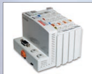
Switch module and interface module for all FA 45 sensors for I/O extension with up to eight additional inputs and up to 32 additional outputs. Connection to vision sensor via RS422.
