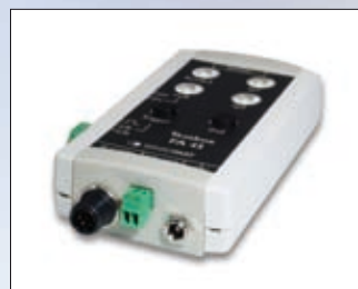
Demonstration and text box for all FA 45 models. Enables test mode with simulation of inputs (trigger or similar) and display of outputs as well as power supply of vision sensor. All I/Os are through-wired, so parallel operation with control system possible.
