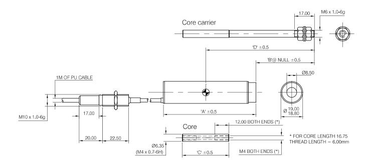
A = Body lengthB = Carrier Protrusion From Front Face at Mid Range (null)
