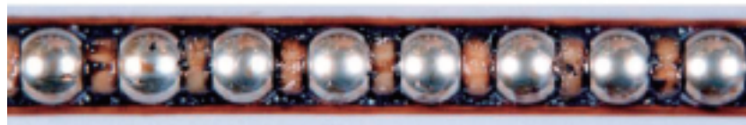
Ball cage after running 8,000 km (Test stop)
