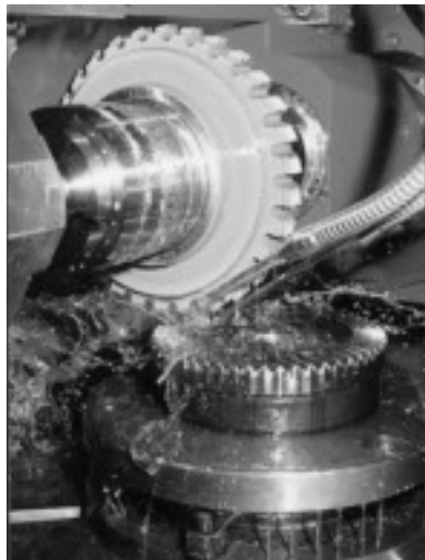
CNC Machining of a PowerTRUE™ right angle gear
